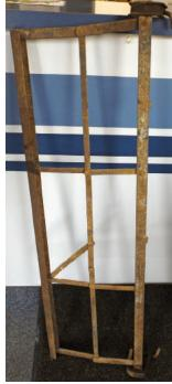
tirely of metal. It measures 46 inches long by 13 inches wide when fully extended out. The item has channel irons on the long sides and flat iron in between that are riveted together to allow it to be fully collapsed together when not used (the angled piece in the above picture can be unhooked, which will allow the piece to
